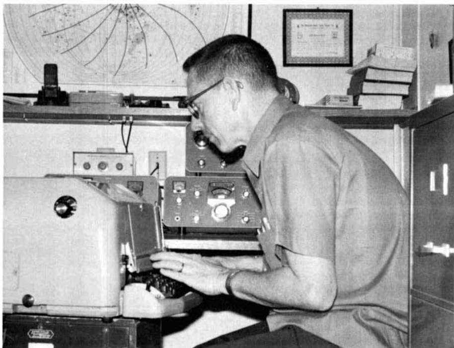
Author W3VF using the variable-speed Kleinschmidt RTTY machine at his station in Pennsylvania.
